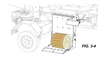
**NOTICE** The log must be less than 24" long, 27" in diameter, and 300 lbs.
