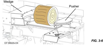
6. Lower the log lift platform as stated in Step
