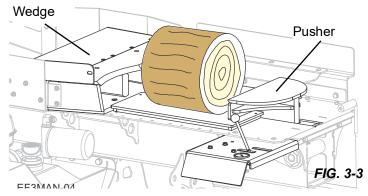
3. Position a log onto the log lift platform.
