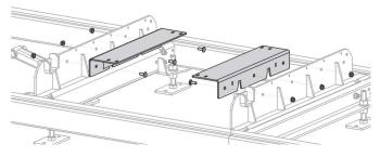
**STEP 3:** Mount the CookieMizer with 5/16" fasteners as shown here.
