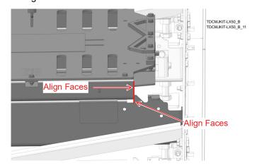
**STEP 5:** Use 5/16" fasteners to secure the clamps to the CookieMizer.
