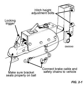
3. Cross the safety chains underneath the hitch and hook to the vehicle. The chains should be connected so that there is still slack in the chains when the vehicle is turned sharply in either direction.
