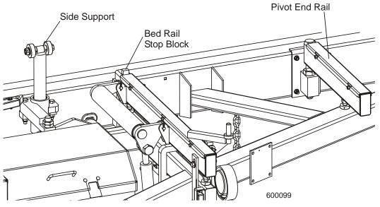
**Rev. A5.00+:** Setup the board return table for operation.
