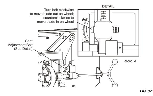
To move the blade out on the blade wheel, turn the cant adjustment bolt clockwise. To move the blade in on the blade wheel, turn the bolt counterclockwise.
