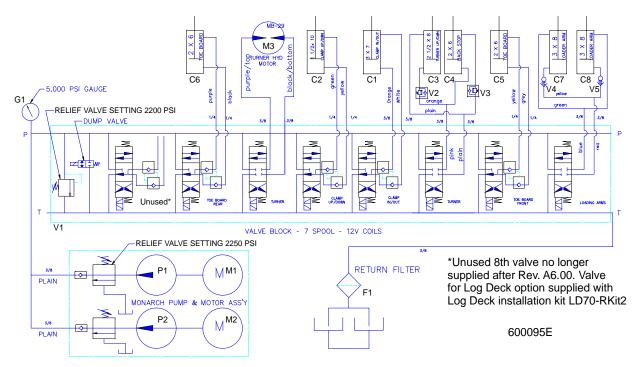
FIG. 8-1 HYDRAULIC SCHEMATIC (DC REMOTE MODELS)
