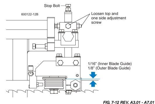
Measure the distance between the flange on the inner blade guide roller to the back edge of the blade. This distance should measure 1/16" (1.5 mm). Adjust the roller back or forward if necessary.
