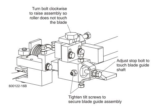
adjust the stop bolt so it touches the end of the blade guide mounting shaft.
