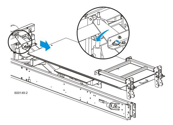
4. Remove the four leg pins and pivot the legs toward the ground. Replace the leg pins.
