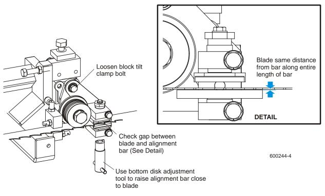
**Rev. A7.02 - A8.00**: To adjust, turn the tilt adjustment jam nuts to pivot the block assembly until the alignment bar is parallel to the blade. Retighten the jam nuts. Repeat for the second blade guide assembly.
