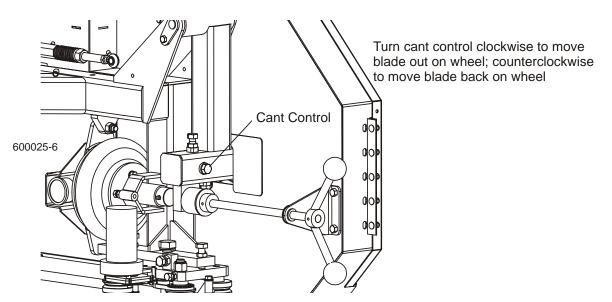
**10.** Check the position of the blade on the drive-side blade wheel. The blade should be positioned on the wheel as described for the idle-side blade wheel. Adjust the drive-side blade wheel if necessary.
