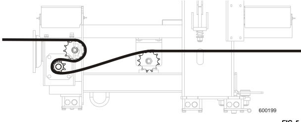
See Figure 5-17. Refer to the diagram for power feed chain routing instructions.
