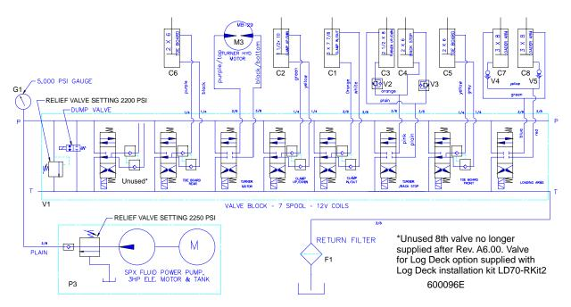
FIG. 8-2 HYDRAULIC SCHEMATIC (AC REMOTE MODELS)
