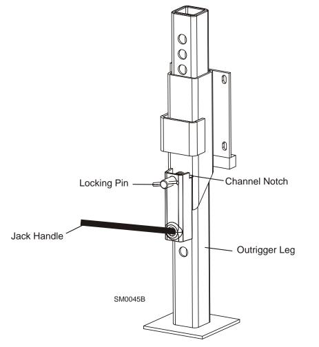
FIG. 3-14. OUTRIGGER ADJUSTMENT.
