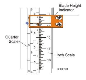
The scales are attached to the frame and move up and down with the saw head. The blade indicator, used to read the inch and quarter scales, remains stationary.
