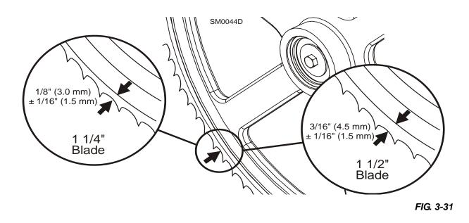
5. Use the cant adjustment bolt to adjust where the blade travels on the blade wheels.
