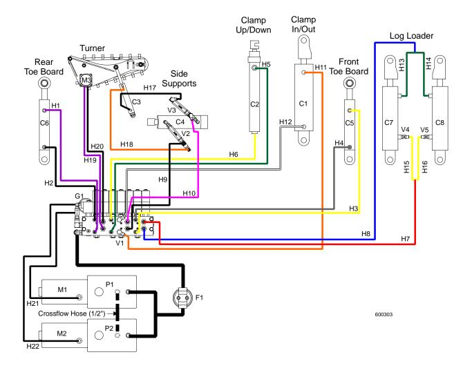
FIG. 8-3 HYDRAULIC LAYOUT DIAGRAM (DC ONLY).
