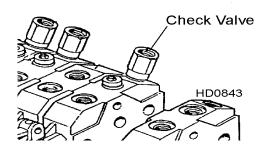
Bad check valve (results in one of the toe boards experiencing down-creep) Check the release valve as instructed above. If the release valve is good, replace the high-pressure hydraulic check valves (A12869) located on the pump.
