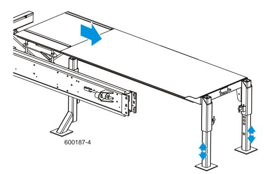
Rev. A3.01 - A4.01: Setup the board return table for operation.
