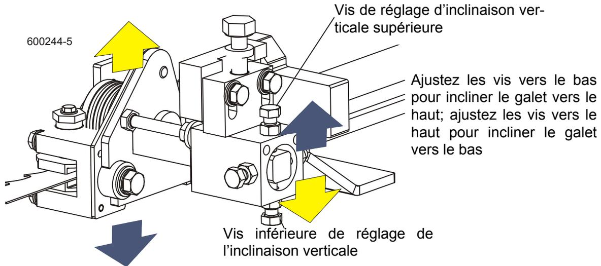
**FIG. 7-9 (GALET/BLOCS DE HAUTE PERFORMANCE ILLUSTRÉS)**
