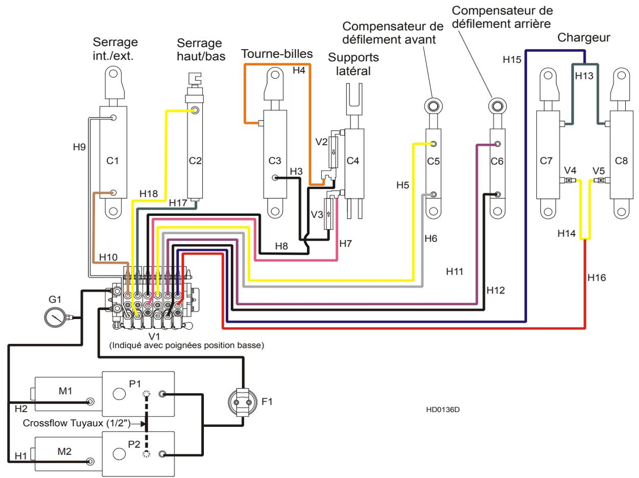
**FIG. 8-2 DIAGRAMME DE LA DISPOSITION HYDRAULIQUE**
