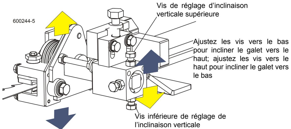
**FIG. 7-38 (GALET/BLOCS DE HAUTE PERFORMANCE ILLUSTRÉS)**
