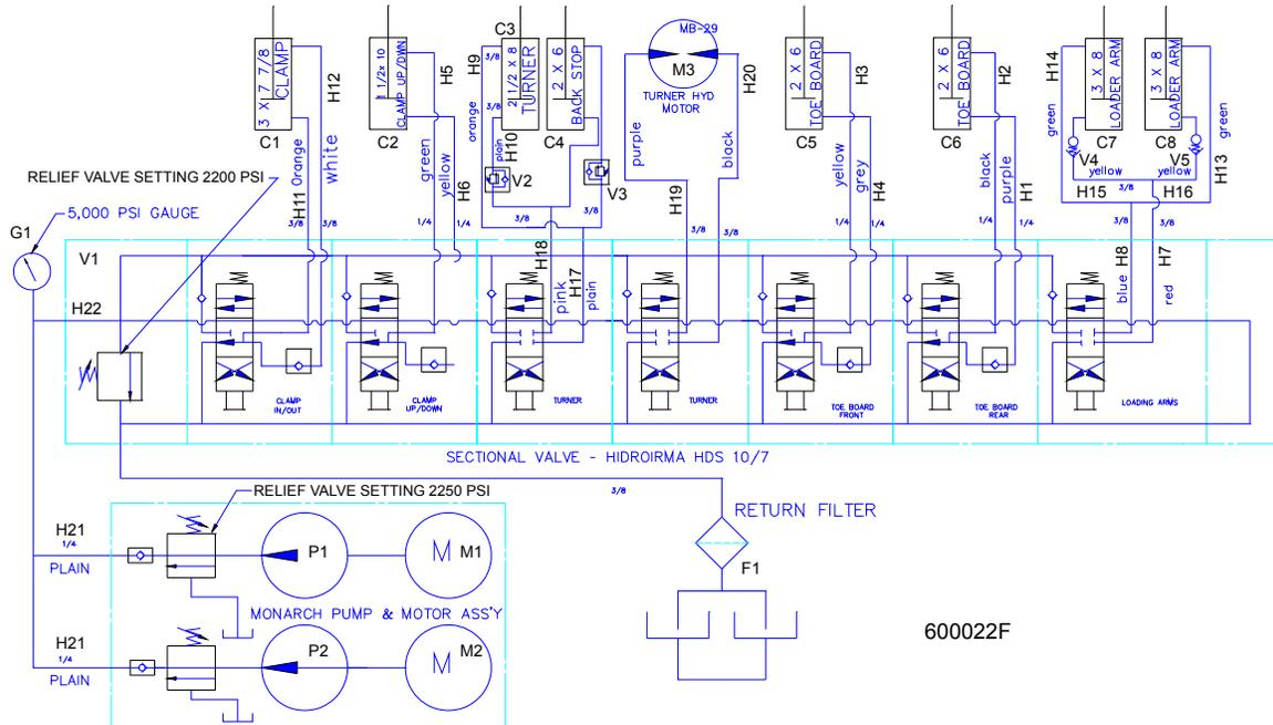
FIG. 8-1 SCHÉMA HYDRAULIQUE
