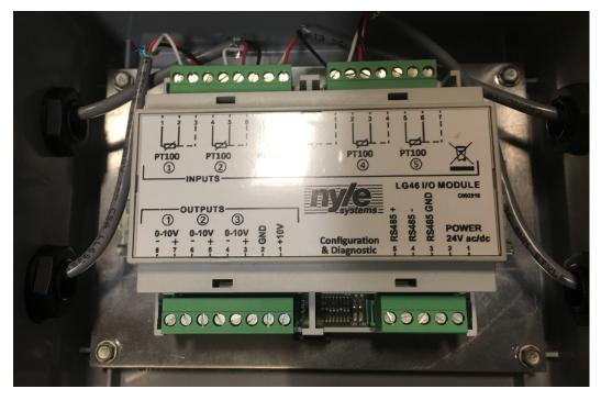
The wood probes are wired in as follows: White goes to 1 Red goes to 2 Black goes to 3 Then repeat for the last 3 probes. An example is shown below.
