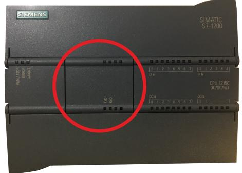
If there is a plastic insert where the above picture is labeled TxD and RxD, interfacing with the probe packages should be as simple as replacing the plastic insert with the provided snap-in module, and wiring the leads from the kiln into the snap in module, like this: Black to M, white to T/RA, white jumper between TA and T/RA, green to T/RB, and a green jumper between T/RB and TB.
