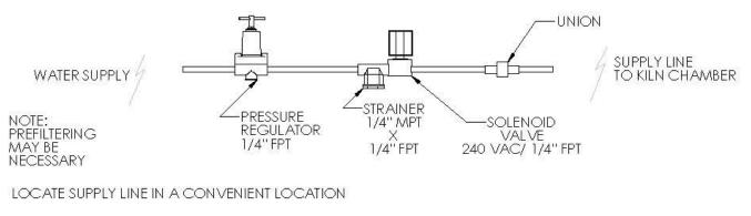
ELECTICAL CONNECTIONS: WIRE THE SOLENOID VALVE BACK TO NYLE ELECTRICAL PANEL AND CONNECT TO TB1 16 AND 10
