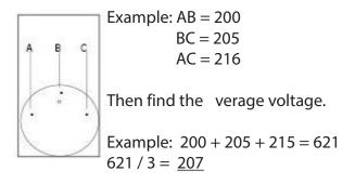
Find the difference between the average voltage and the measured voltages for AB, BC and AC. This is called the standard deviation. The highest number is your maximum deviation.
