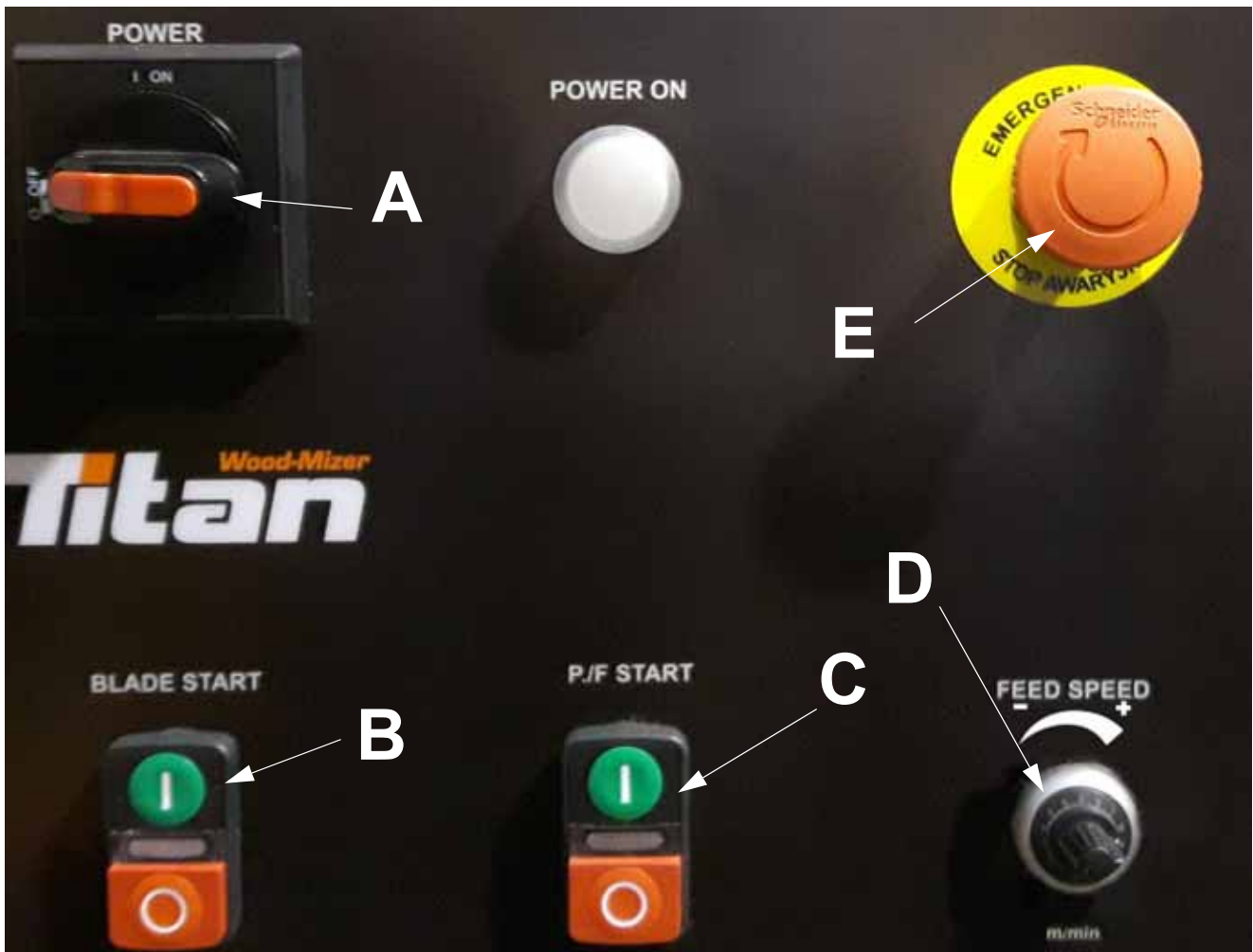
FIG. 3-6 SWITCHES ON THE CONTROL PANEL
