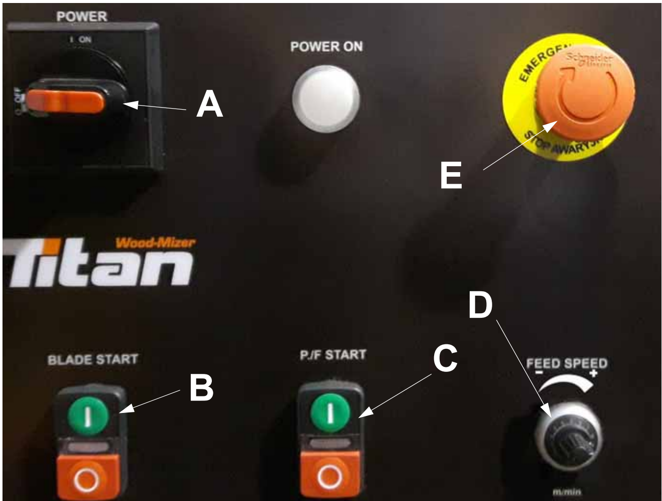
FIG. 3-3 SWITCHES ON THE CONTROL PANEL
