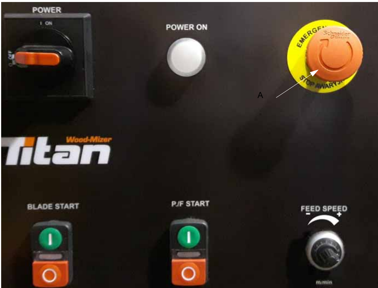
FIG. 4-14 SWITCHES ON THE CONTROL PANEL
