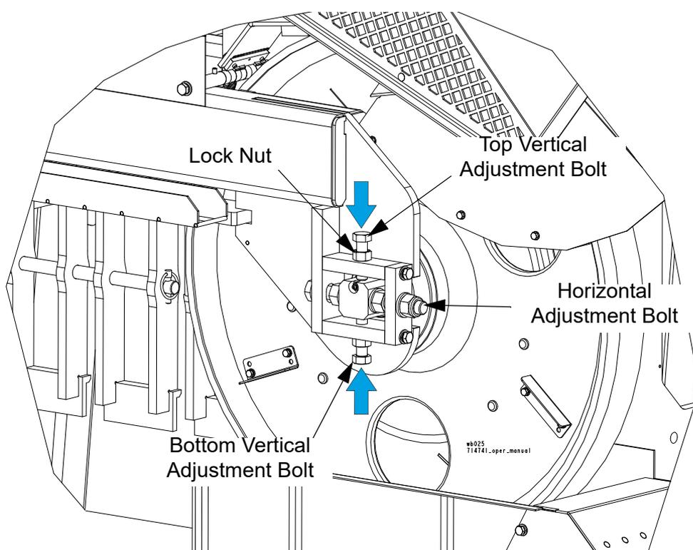
**FIG. 5-8 DRIVE SIDE WHEEL VERTICAL ADJUSTMENT**
