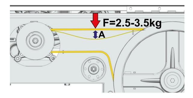
6. To adjust the engine drive belt, use the bolts mounting the engine to the engine mount plate.
