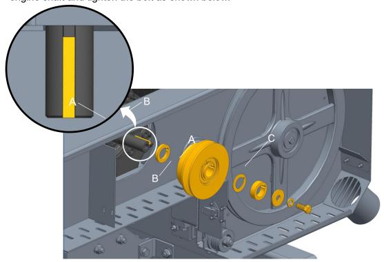
2. Hold the bushing (A) with an adjustable wrench and tighten the bolt (B).
