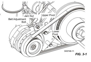
**9.** After the alternator belt has been tensioned, tighten the adjustment bolt jam nut.
