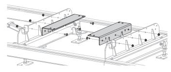
**STEP 3:** Mount the CookieMizer with 5/16" fasteners as shown here.
