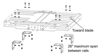
**STEP 2:** Loosely mount the brackets to the bottom of the CookieMizer at the outermost slots.
