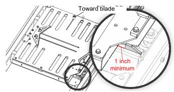
**STEP 3:** Place the flat mounting plates on the inside of the CookieMizer at the outermost slots.
