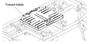
**STEP 3:** Place the flat mounting plates on the inside of the CookieMizer at the outermost slots.
