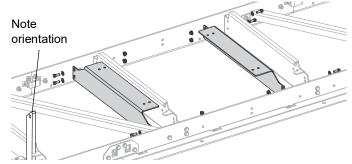
**STEP 3:** Mount the CookieMizer with 5/16" fasteners as shown here.
