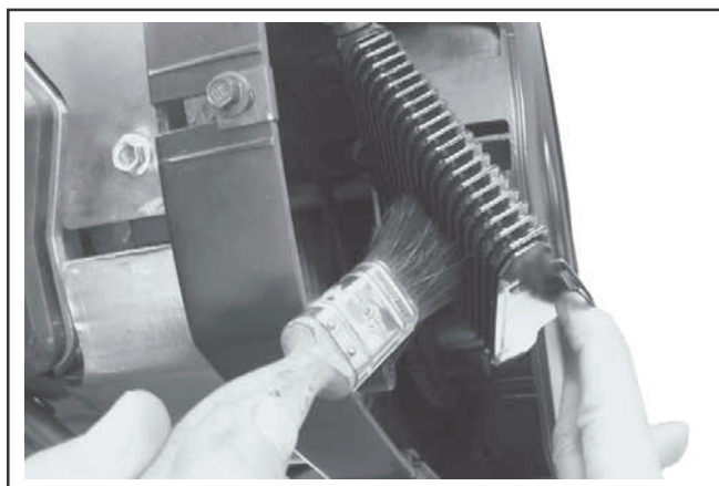
Figure 18. Cleaning Underside of Oil Cooler.
