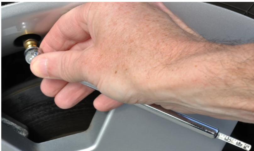
COMMON TIRE PRESSURE GAUGES
