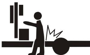
**DANGER!** Keep all persons out of the path of moving equipment and logs when operating sawmill or loading and turning logs. Failure to do so will result in serious injury.
