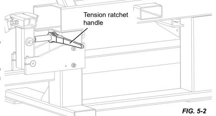
Tighten the tension by ratcheting the device handle until the pivot arm is touching the stop bolt.
