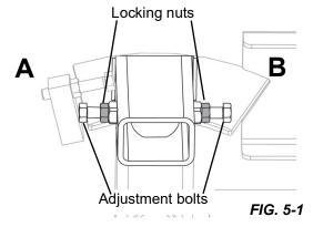
the blade AWAY FROM THE BLADE GUIDE BEARING.
