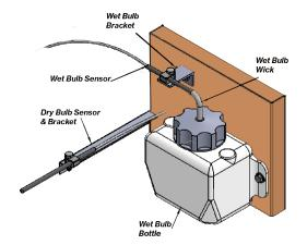
**Step 5:** Slide 2" (50mm) of the wick into the sensor.
