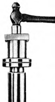
Fig. 8. Press Small Bearing on Shaft
