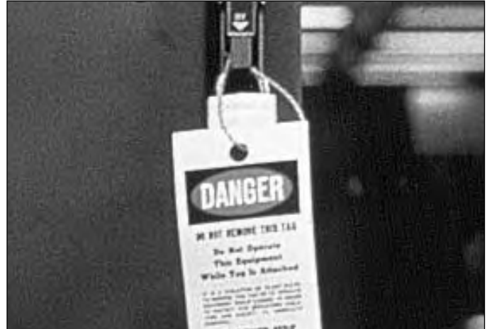
Turn off power, lock controls and tag
