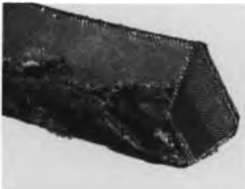
Cover Fabric Rupture
