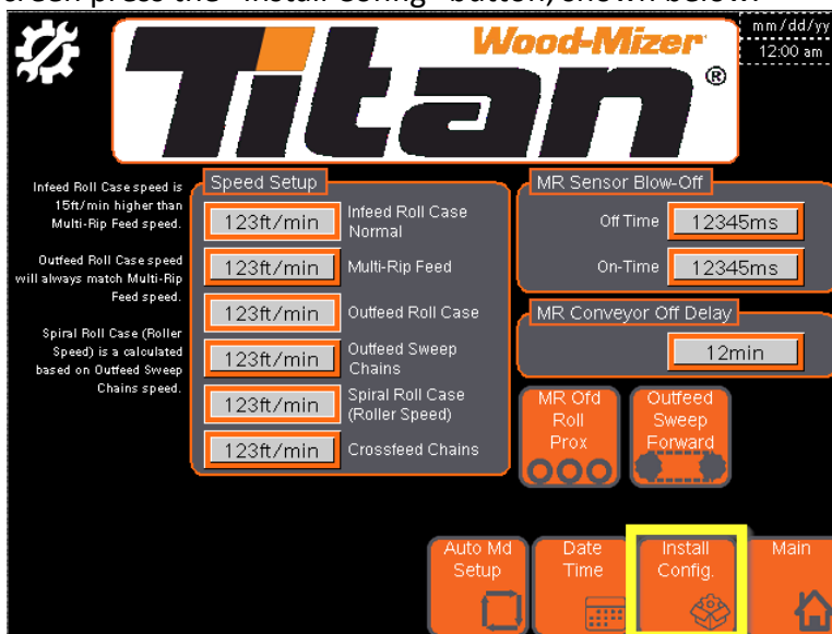
Figure 4 – Setup Screen: Install Config Button
