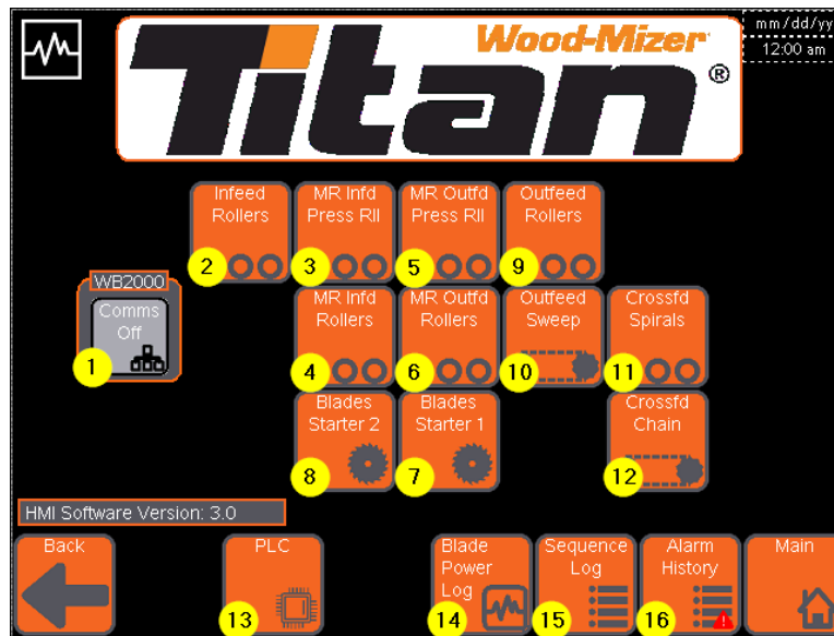
Figure 42 – Diagnostics Main Screen
