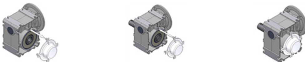
Figure 18: Removal and fitting of the cover cap
