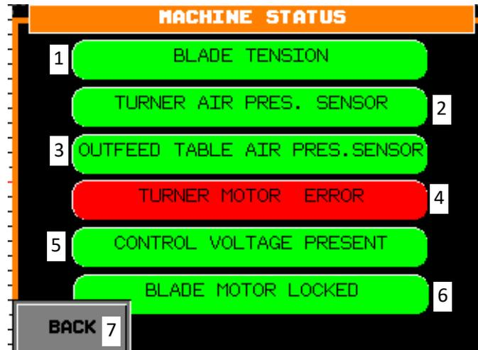
Green colour: the machine is ready for starting the main motors. Red colour: it is not possible to turn on the blade motors.
