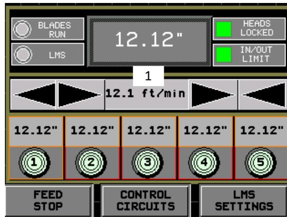
1. When imperial units of measure are selected, the feed rate is displayed in ft/min.
