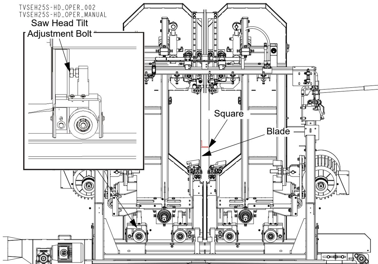
2. Measure the distances between the blades at the lowest and highest points. If the measurements
