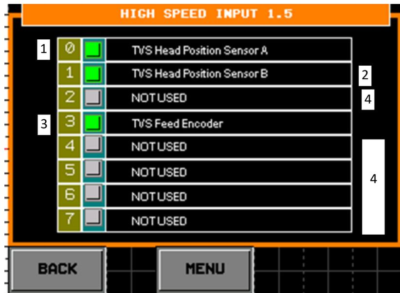
1. TVS saw head position sensor - A,
