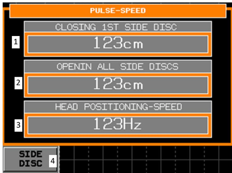
1. Setting the closing position of the first side disk on the outfeed table,
