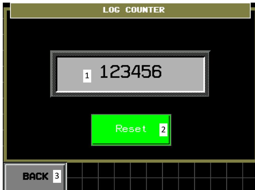
The number of sawn logs is calculated as soon as the feed operation is started (the log is behind the B5 infeed sensor).
