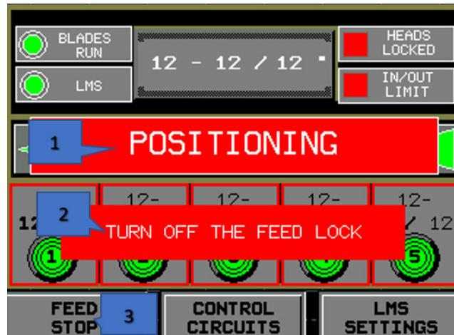
1. This message appears while the saw heads are positioned. Then all position selection keys on the operator panel are locked.
