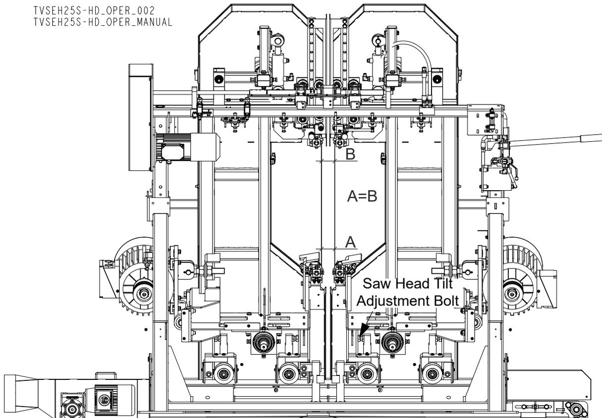
3. Check if the saw heads are perpendicular to the table. Adjust if necessary.
