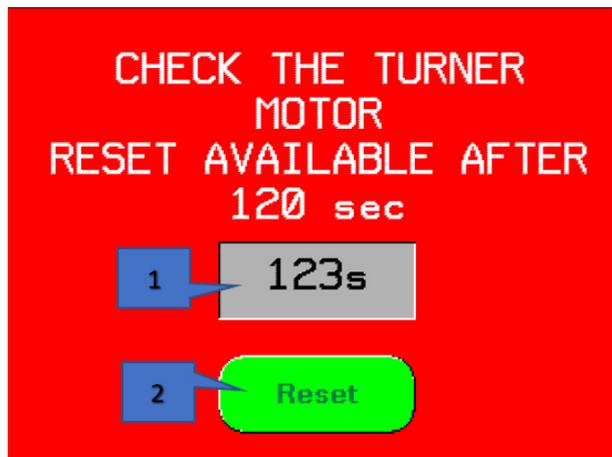
1. A counter that calculates the time since the error occurred. After 120 seconds, the key "2" changes from gray to green allowing the operator to reset the motor controller.
