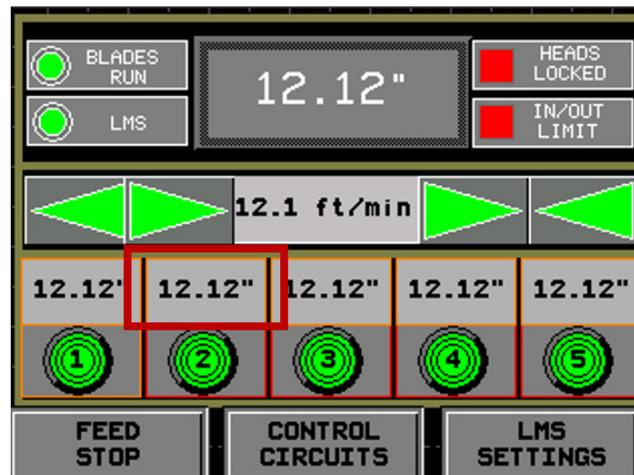
After pressing any of the five fields (shown above) with stored cutting width value, a window will automatically appear where the operator can enter the real cutting width.
