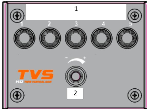
1. Five programmable keys the operator can use to automatically set the desired distance between the blades
