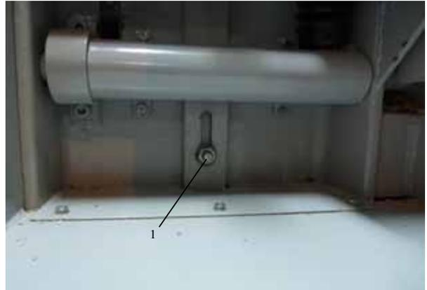
1. Nut of the connector of the upper spindle support with the motor support
