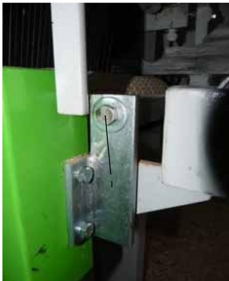
1. Workpiece guide adjustment bolt
