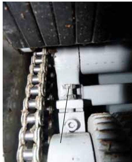
1. Pressure roller chain tensioning bolt
