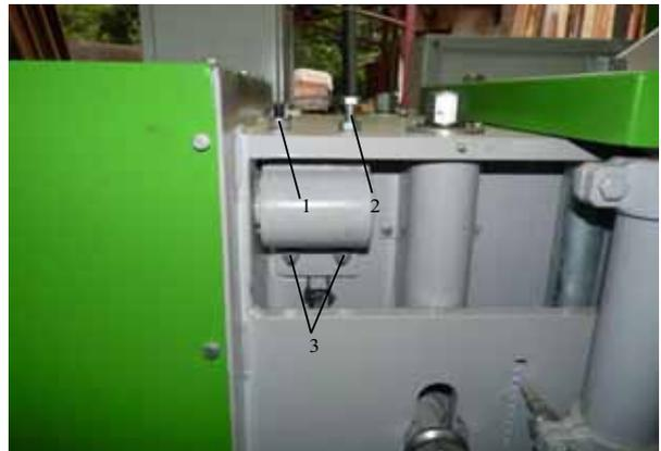
1. Tensioning nut of the indirect chain
