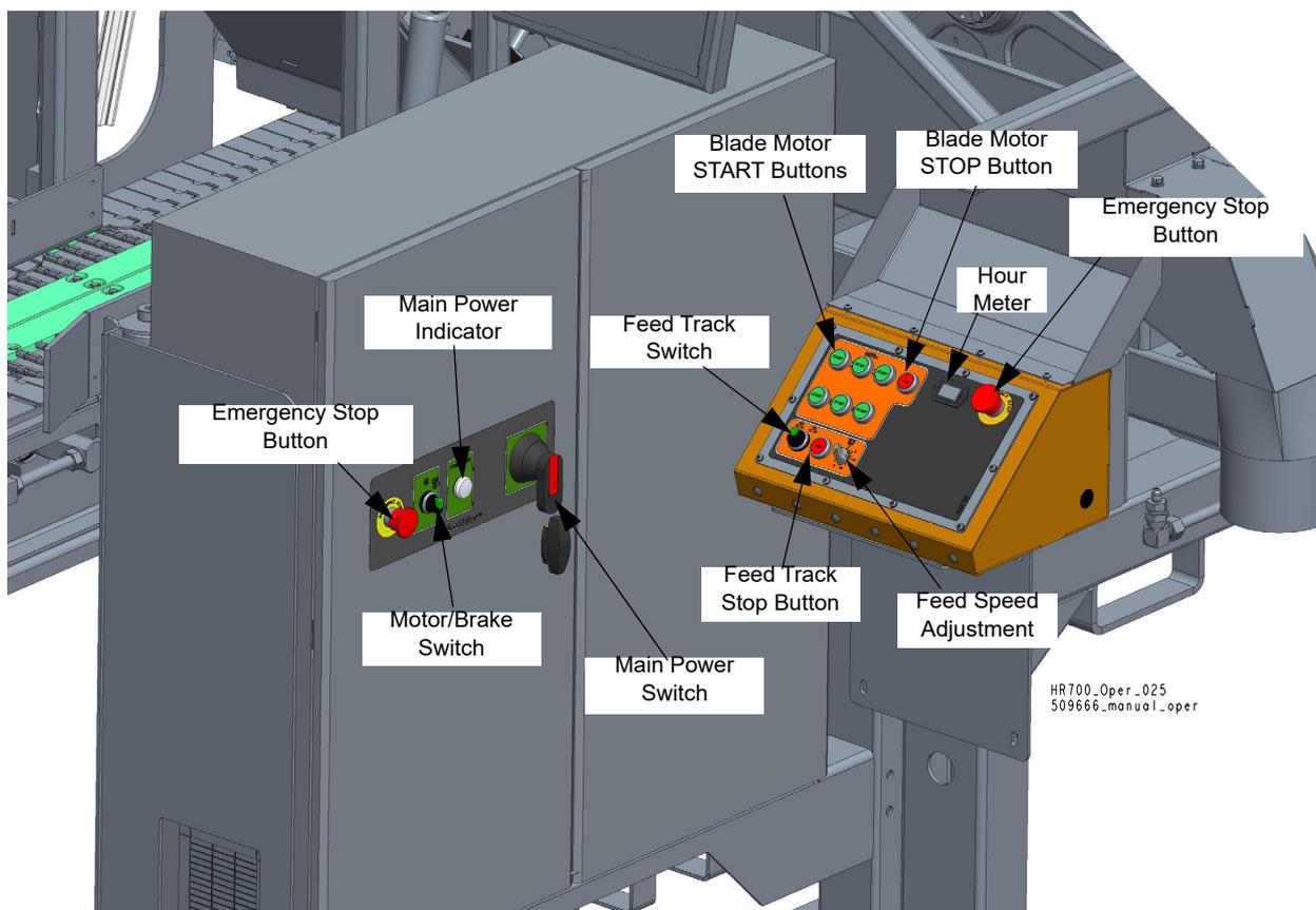
**FIG. 2-1 CONTROL PANEL AND MAIN ELECTRIC BOX**
