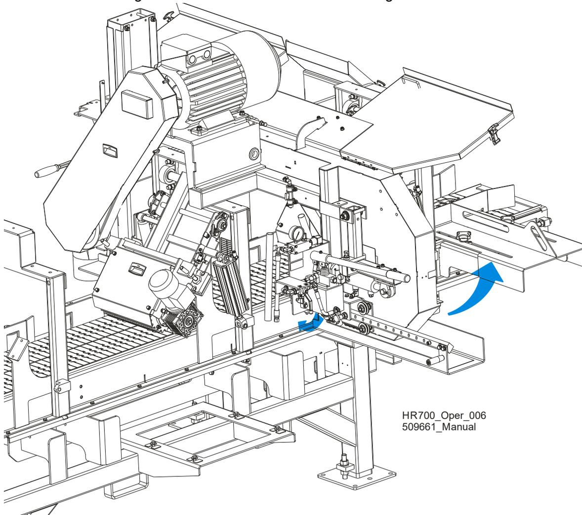
Install a new blade around the two blade wheels so that the teeth located between the blade guide assemblies point to the drive side of the machine. Make sure the teeth are pointing the correct direction.
