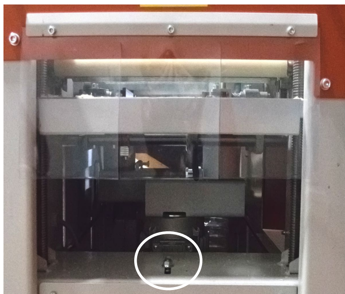
Outfeed view, chain adjustment sprocket lock nut - use 17mm wrench FIG. 5-7
